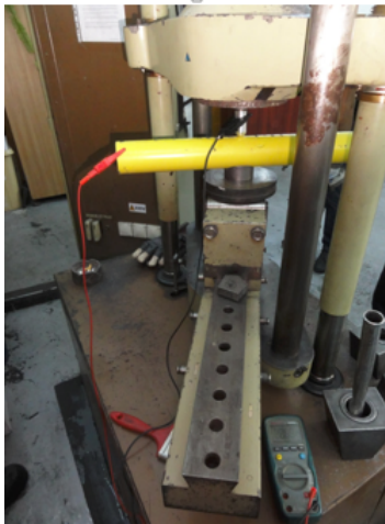
Fig.11. Detail of the installation for determining the insulation resistance
